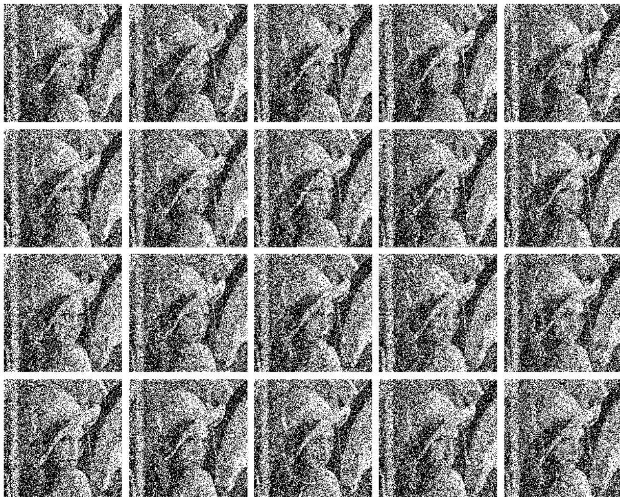
Comparing the original grayscale image to the spike matrix, it can be found that the spike matrix is very close to the contour of the original grayscale image, which shows the superiority of the Poisson encoder.
