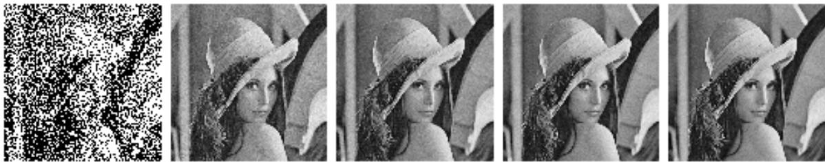
It can be seen that when the simulation is sufficiently long, the original image can almost be reconstructed with the superimposed images composed of spikes obtained by the Poisson encoder.
